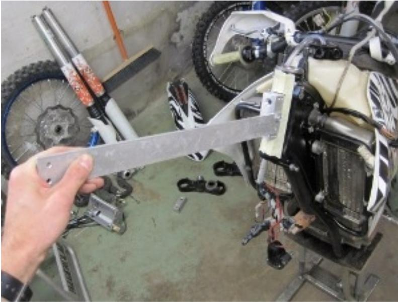
**6:** Mark where the holes goes. From the edge of the brackets to the holes is 16 mm, so at least 16 mm from your marked line. You can use the plate (MRSP) to extend the frame bracket. In the picture, I screwed a longer bar to clearly see where “straight” is. Measure this carefully, and mark two small dots in the center of the holes.
