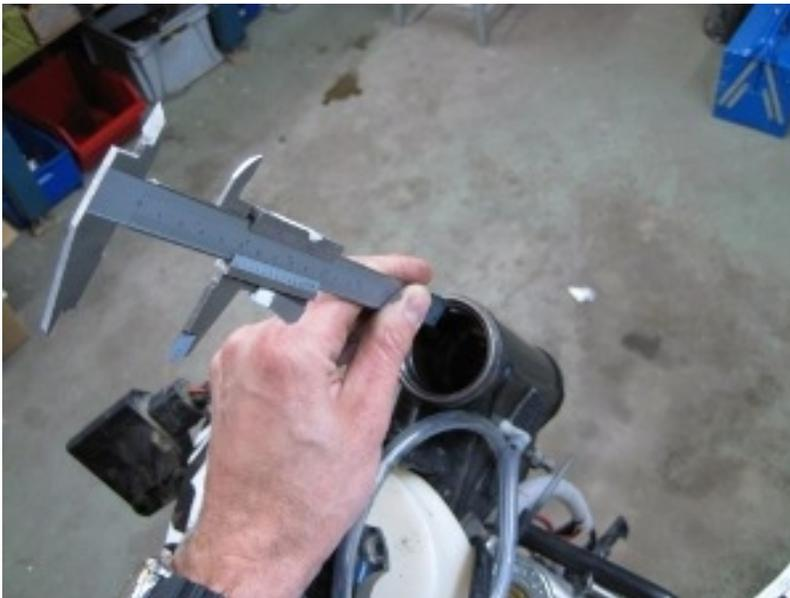
Measure from the inner frame bracket to the edge of the steering tube. Remove the bracket.
