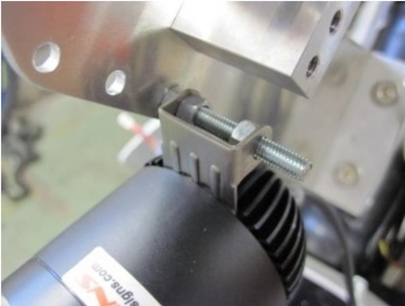
First, screw the M5x40 from the right and tighten with one nut. Install the first ear of the LED holder with two nuts between. Adjust angle and tighten the second one from the right.
