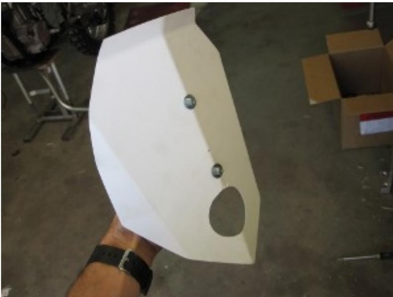
Tighten it so the metal plate meets the fairing, but not too much, glass fibre cracks if you're not careful. Then attach the brackets to your MRS plates and adjust, so the light lines up with the fairing hole.
