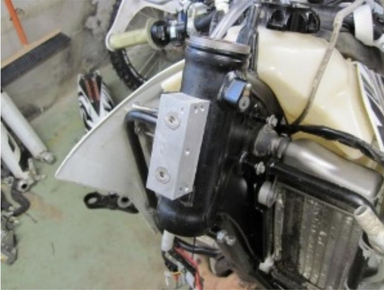
**7:** Install the inner frame bracket together with the outer one, creating a sandwich with the frame between. You can "glue" the inner to the frame with silicon. That way you can later remove the outer frame bracket with the inner one still attached. You should end up with a complete frame bracket. Check that the bracket is straight several times and tighten the screws with 30 Nm.
