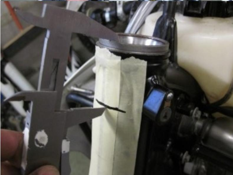
Use this measurement for placing the outer frame bracket edge. Now do this again from the bottom to be sure.
