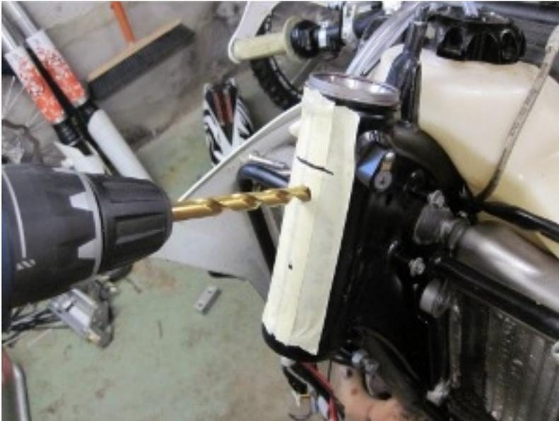
Use a center punch, and drill small holes, then widen them to 10 mm. The 2 extra mm is for adjusting, and also if you crash this will work as play.
