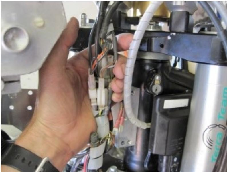
Install everything you need on the handlebars; ODO-meter remote, roadbook-remote, starter, kill switch etc. Try to bring them together in the middle, and down. That way, when you turn the handlebar, the cables don't stretch.
