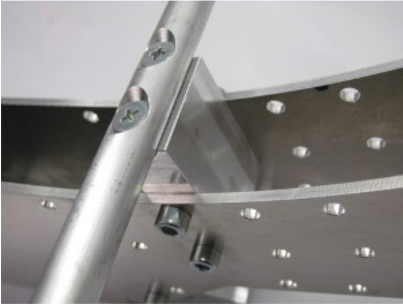
**10: Roadbook holder.** Tilt the steering to one side, and roughly measure where you want the roadbook holder. Take a bracket with suitable length (MRSBxx) and install the bar (MRSB) using two M5x20.
