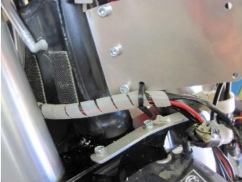
Here's the wiring harness on my bike. It goes under and up inside the two plates.
