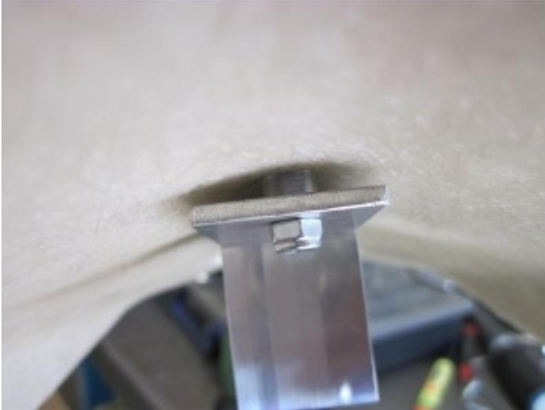
Screw that plate to the fairing using two M5x16 allen heads with washers on the outside and plastic spacer between, in this order:
