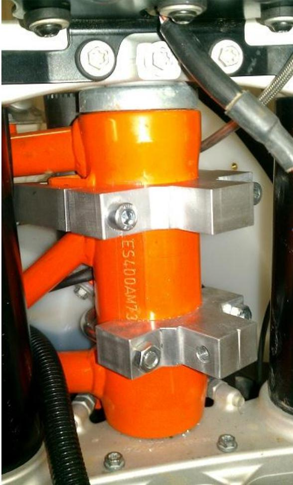
Installation is almost as easy as it looks. The u-shaped part of the bracket is positioned inside the slightly u-shaped part holding the coolant expansion tank. It may be necessary to file a groove in order to fit the U-shaped part snugly against the steering head. After getting the U in place, simply add the lower frame bracket and do up the lock nuts. Position the bracket in accordance to the top frame bracket to ensure straightness.
