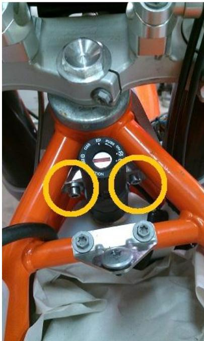
Loosen the bolts for the ignition barrel. Replace the bolts with the supplied M6 Allen bolts. We have supplied 3 different lengths as there are great differences in production regarding the brackets for the barrel.
